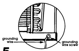
**D** Loosen, but Do Not remove grounding wire screw. Disconnect grounding wire.
